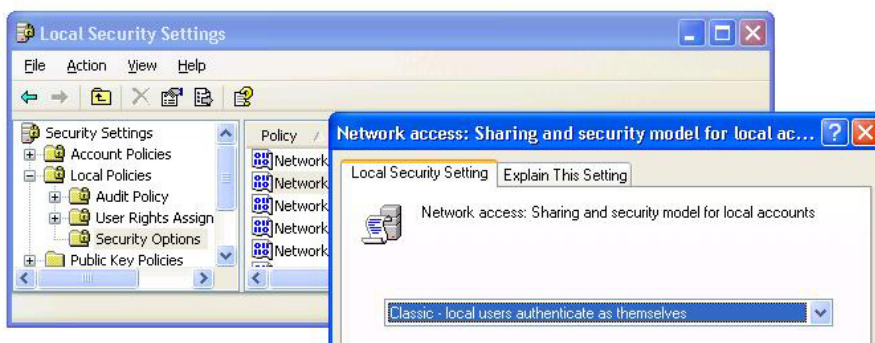
Figure 13.3 You can use the secpol.msc MMC snap-in on Windows XP SP3 to enable PowerShell remoting to access this machine. The displayed policy item must be set to Classic for remoting to work.
