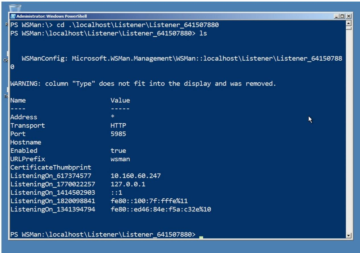
Figure 7.5: Checking the newly created WinRM listener
