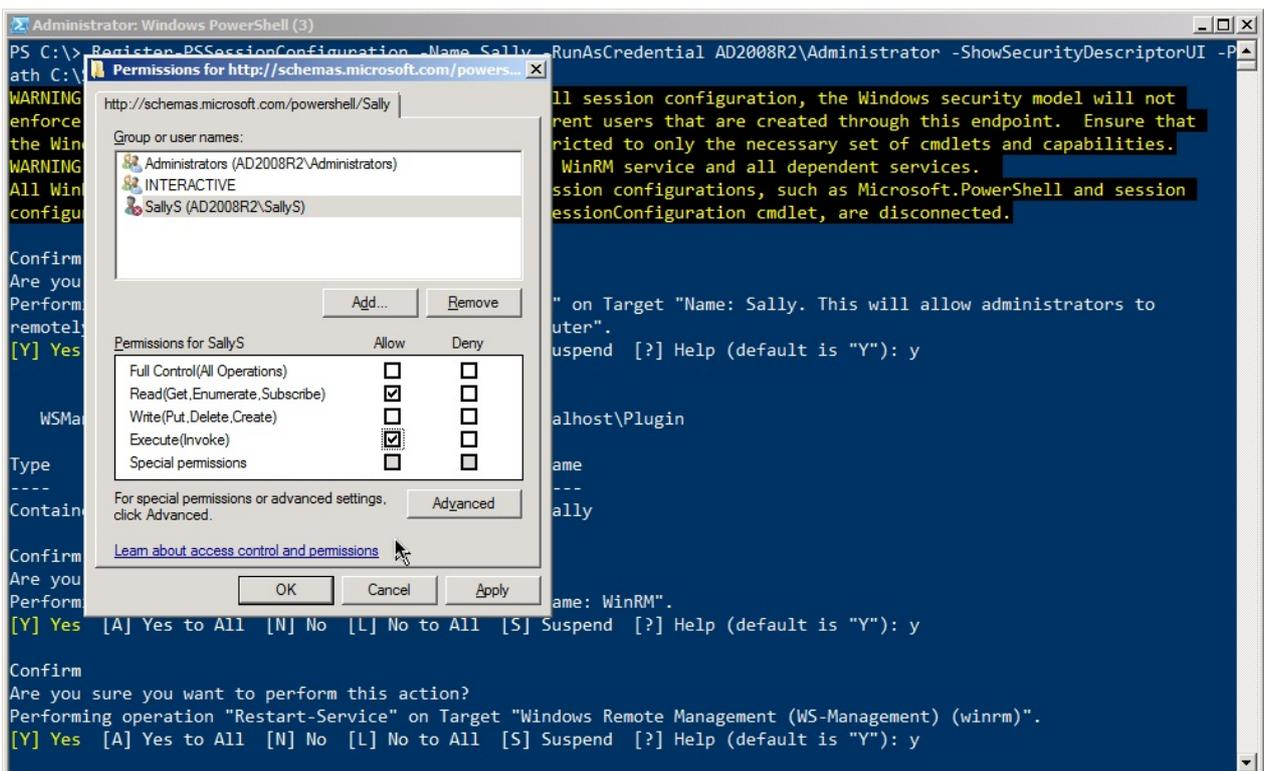
Figure 3.7: Setting the permissions on the endpoint
