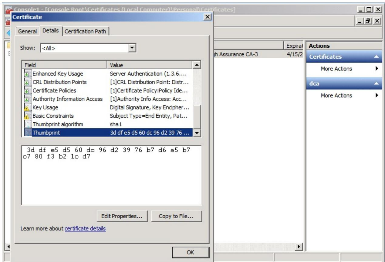
Figure 2.14: Obtaining the certificate's thumbprint
