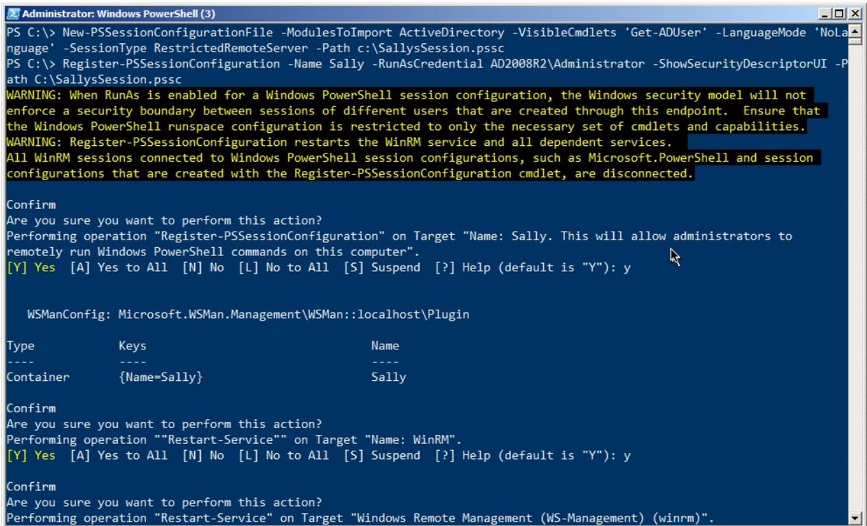
Figure 3.6: Creating and registering the new endpoint
