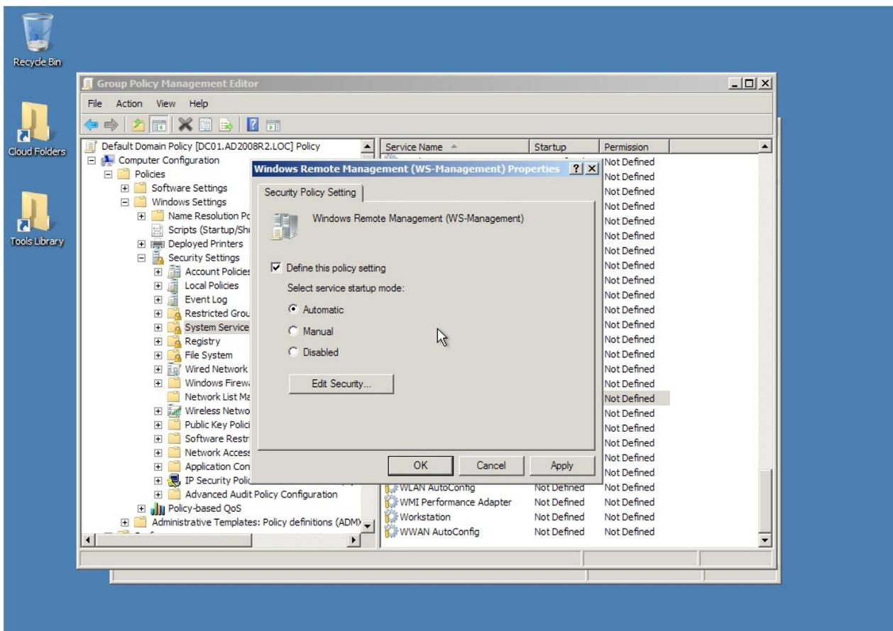
Figure 7.2: Setting the WinRM service start mode
